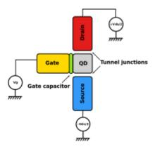
The simplest device in which the effect of Coulomb blockade can be observed is the so-called single electron transistor. It consists of two electrodes known as the drain and the source, connected through tunnel junctions to one common electrode with a low self-capacitance, known as the island. The electrical potential of the island can be tuned by a third electrode, known as the gate, capacitively coupled to the island.
