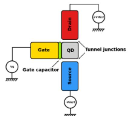
The simplest device in which the effect of Coulomb blockade can be observed is the so-called single electron transistor. It consists of two electrodes known as the drain and the source, connected through tunnel junctions to one common electrode with a low self-capacitance, known as the island. The electrical potential of the island can be tuned by a third electrode, known as the gate, capacitively coupled to the island.
