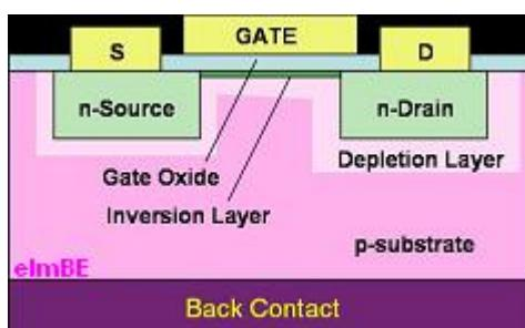
MOSFET(Metal-Oxide Semiconductor Field Effect Transistor)
